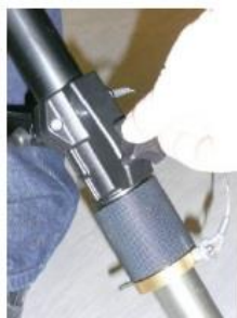
Untighten screw and set the spirit level horizontally
