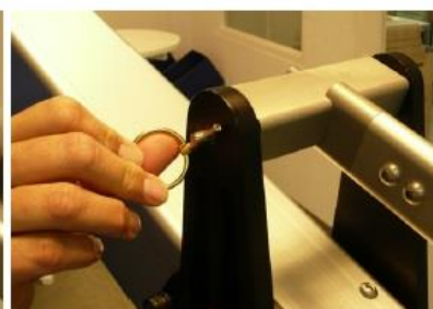
... and secure with quick pin
