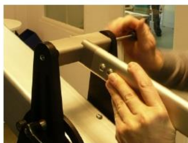
Remove tilt axis from bull stand head and place Movie Jib into it (2 center pins meet 2 holes)
