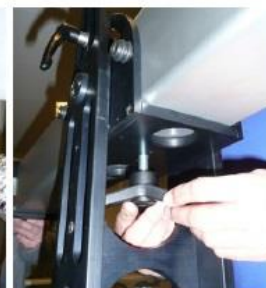
Fixing screw to be inserted from bottom side
