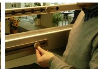
Adjust front extension parallel as requested and fix both knurled screws in the related notches
