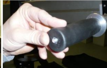
To remove handle push button ...
