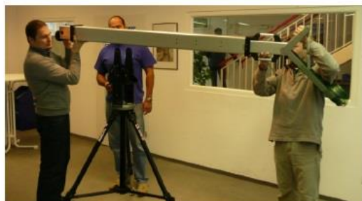
Remove tilt axis from bull stand head and place Movie Jib into it (2 center pins meet 2 holes)
