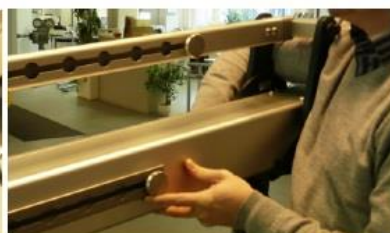
Adjust front extension parallel as requested and fix both knurled screws in the related notches
