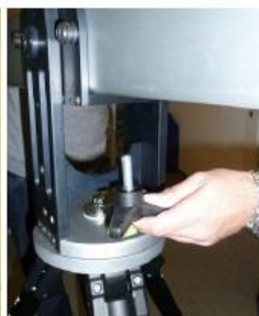
Fixing screw to be inserted from bottom side
