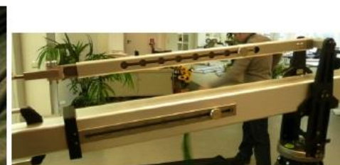
Adjust front extension parallel as requested and fix both knurled screws in the related notches
