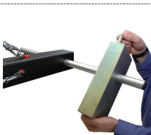
53. Gewichte aufladen. "Kran in die Waage bringen" / Load up the counterweights for taring the crane, secure weights on tubes with securing clips
