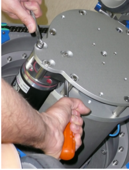
Support motor underneath pulley with screwdriver, remove 3 hexagon screws
