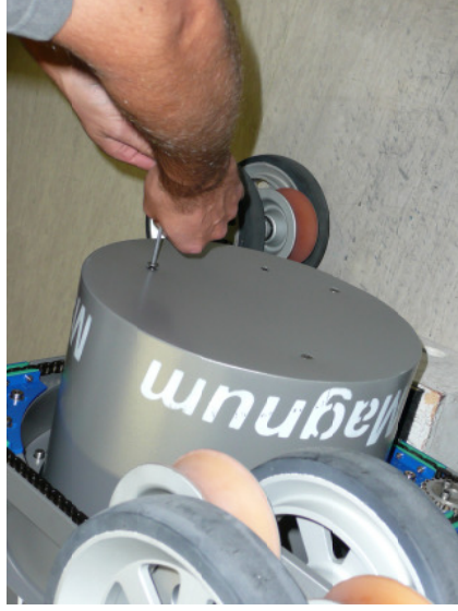
Unscrew the noise reduction cover,
