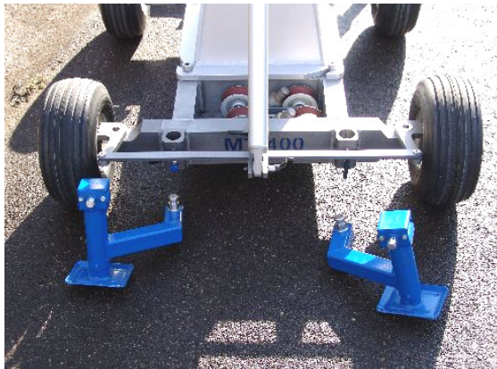
Fig. 7: Operation with levelling legs or tracks
