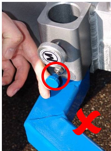
Fig. 8: Incorrect position of the locking pin
