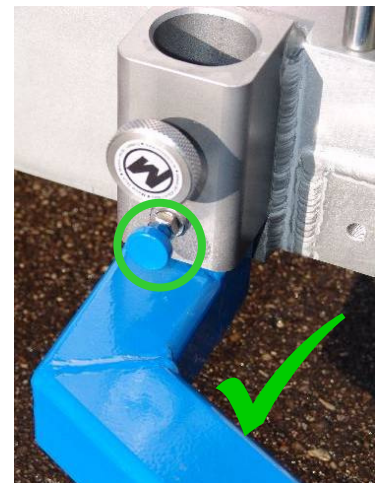
Fig. 10: Correct position of the locking pin
