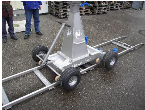
Fig. 13: Base on a track system on level surface
